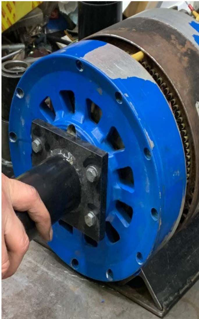
Connect airline to foot pump and slowly engage hydraulic
