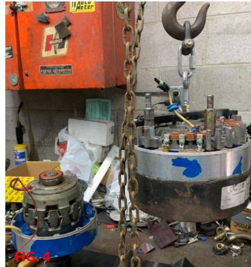
Fig 3,4 – attach TWR harness using large screw bolts to rectifier and lift using a block and tackle
