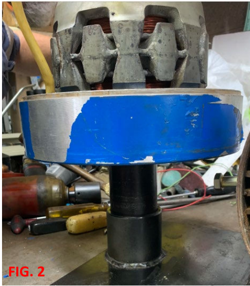
Fig 1, 2 – using shaft of rotor, set rotor/cover into TWR plate stand
