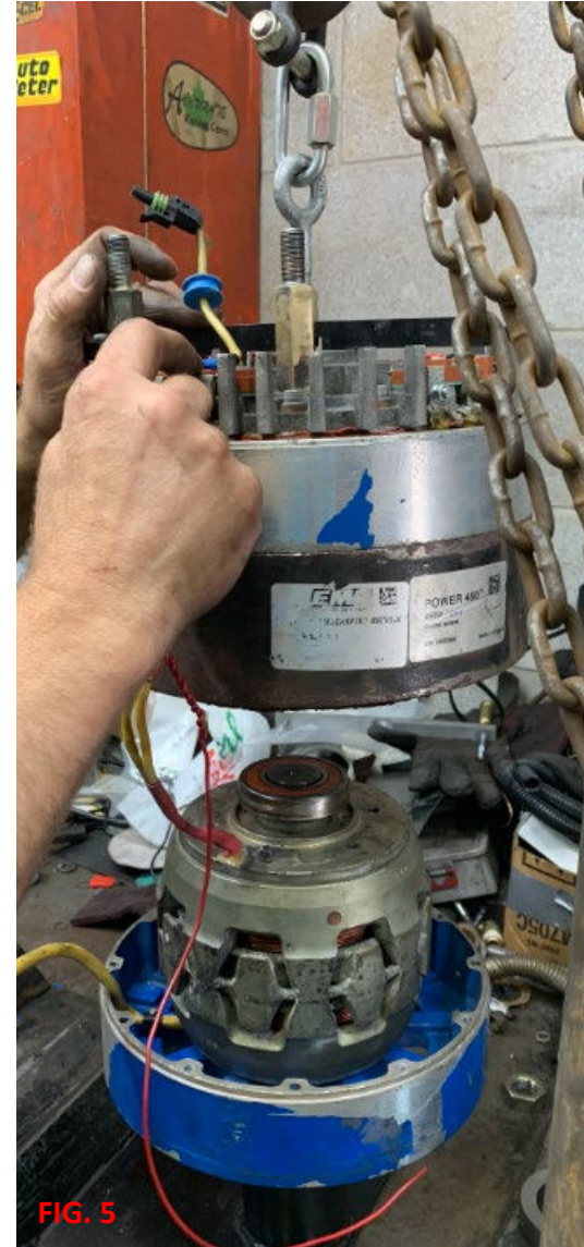
Fig 5 – attach guide wires to help ensure coil wires align
