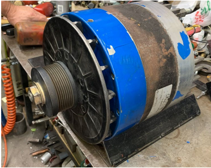
Set unit inside the TWR cradle, remove back cover
