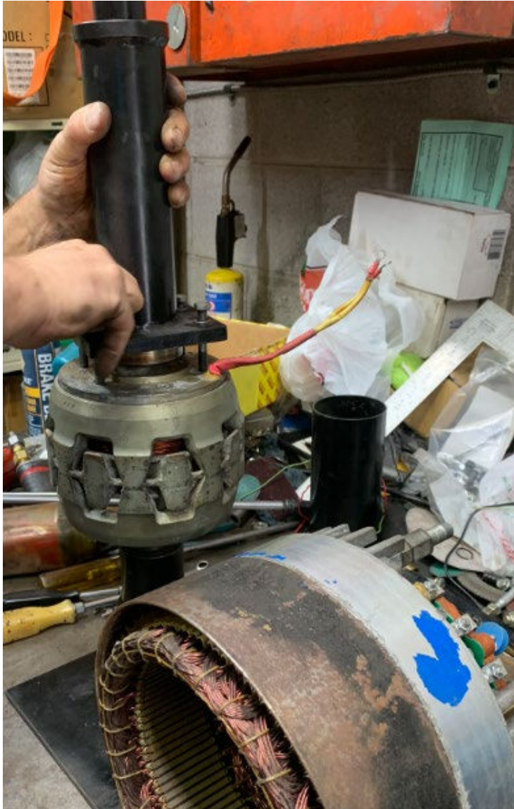
Install TWR Hydraulic Ram over bearing and tighten bolts onto coil
