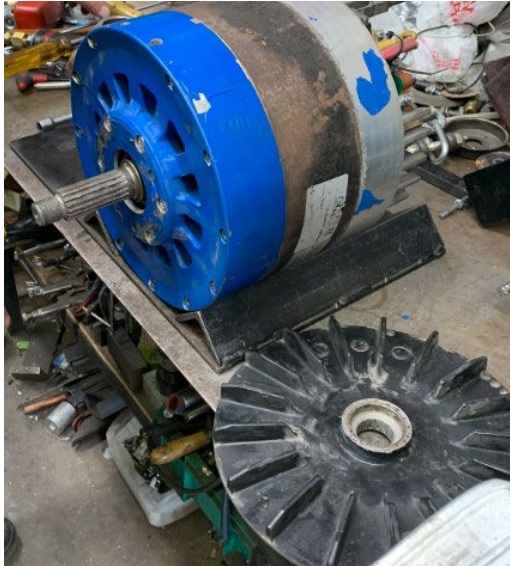
Once pulley is removed, remove fan
