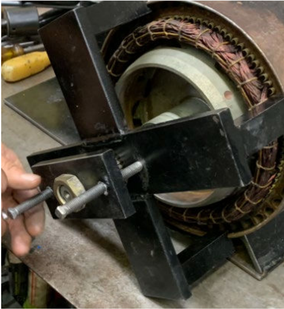
Using TWR Rotor puller, align edge of stator housing with groves in puller, reinstall nut on rotor.
