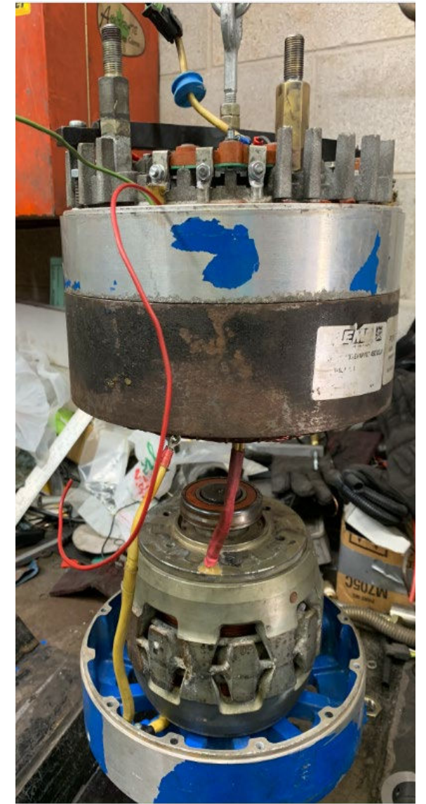
Watching alignment, slowly lower over rotor
