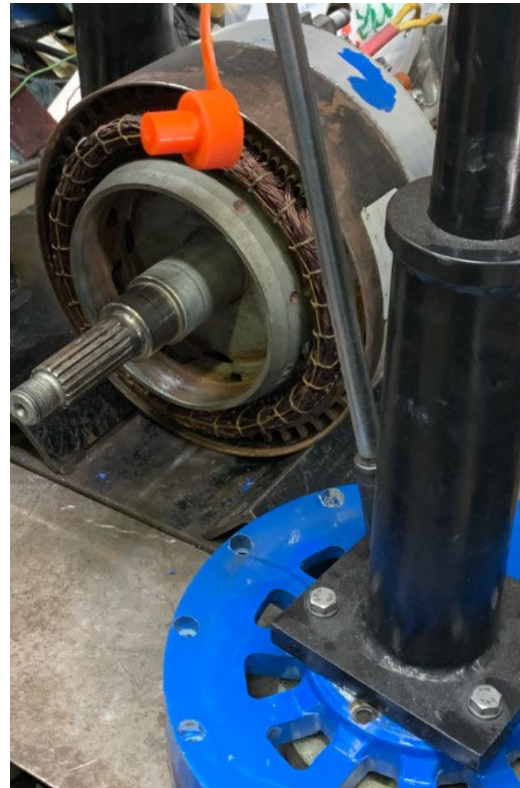
Front cover and bearing will pull away from rotor and stator. Remove Ram Puller from Cover
