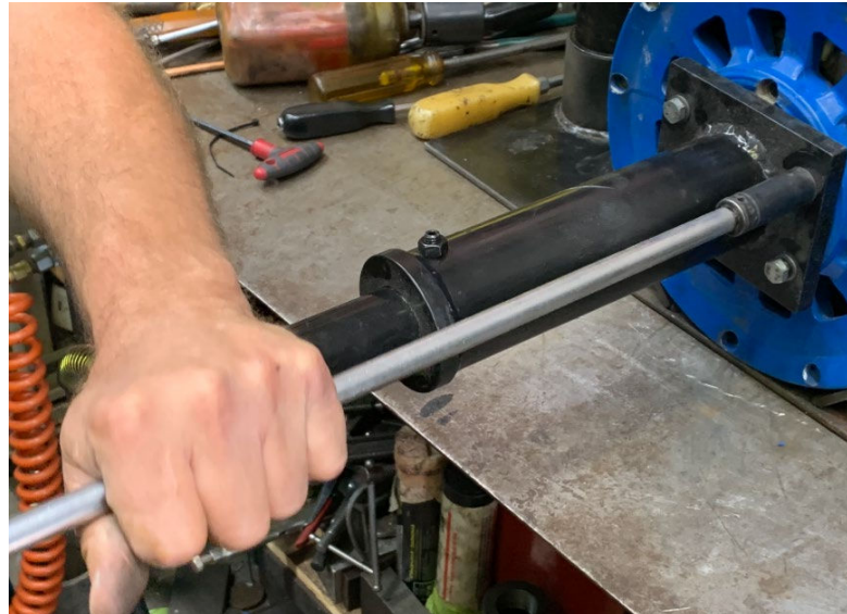
Attach TWR hydraulic ram puller to rotor
